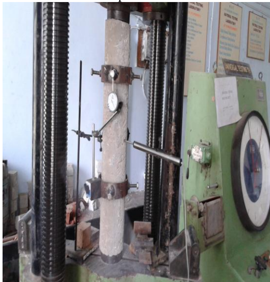
Photo 1. Test set-up for short column
